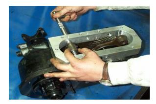
Before installing the other shift rail, pick up the idler gear from the bottom of the case and reinstall the idler gear shaft from the back of the housing. Be sure the thrust washers, two thin spacers and needle bearings have all stayed in place. Tap shaft all the way through, making sure that the notch on the shaft lines up the retainer bolt hole on the back of the case. Reinstall retainer and bolt at this time.
