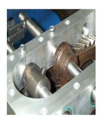
Now, using the original inspection cover, it is time to seal up the case. Make sure there is not any trash or medal shavings in the case. Remove the two bolts temporarily holding the shifter plate to the case. Apply a layer of RTV sealer to the top of the shifter plate. Make sure the detent springs stay in place. Reinstall the inspection cover plate using the 5/16" x 2-1/4" bolts and lock washers (supplied).
