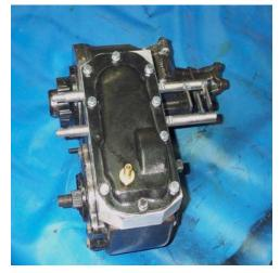
Remove plug in the inspection plate cover. Install the new brass nipple in its place; this is your new vent hose connection.
