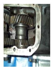
Place the aluminum shifter plate on the inspection cover opening, insuring that the square corner of the plate is on the backside closest to the rear output shaft. At this time, use a bead of RTV sealer to seal the aluminum spacer to the housing. To temporarily hold the spacer in place, use two of the 5/16" x 2-1/4" bolts to keep the spacer from moving while the shift rails are being installed.
