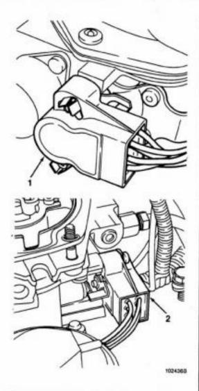
Sensor operation is checked by measuring input and output voltage. Sensor adjustment involves changing output voltage by rotating the sensor to change voltage. Sensor input and output voltage is checked at the sensor wire harness connectors with a voltmeter.
