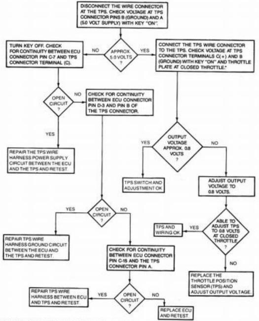
DO NOT UNFASTEN THE SENSOR WIRE HARNESS CONNECTOR. INSERT THE VOLTMETER TEST LEADS THROUGH THE BACK OF THE WIRE HARNESS CONNECTOR TO MAKE CONTACT WITH THE SENSOR TERMINALS.
